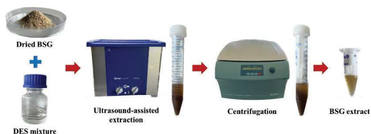
Figure 1: Protocol for the extraction of polyphenolic compounds from BSG.
